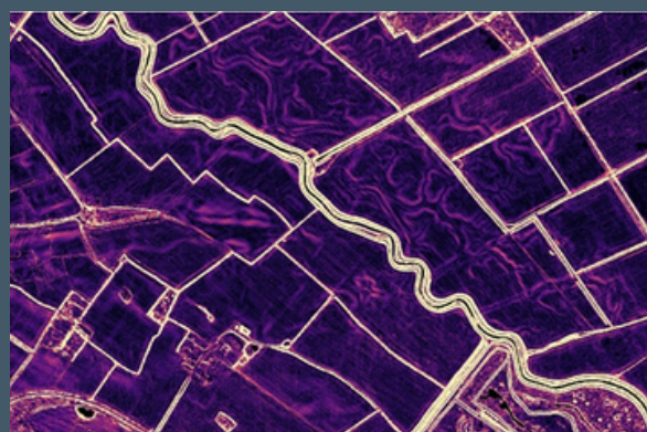
Aerial vs LiDAR images. LiDAR shows lots of small channels and low areas in fields which may be historic wetlands
