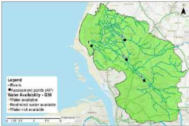
Map 2: water resource availability colours at Q30 for the Alt catchment (high flows)
